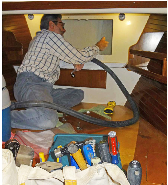
Removing the chain locker center divider
