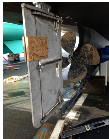
Articulating rudder on temporary installation blocks
