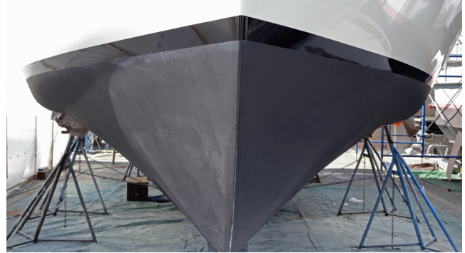
Rounded chine with bottom paint
