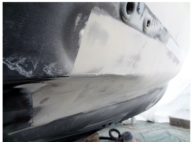
Transition from hard chine to rounded chine
