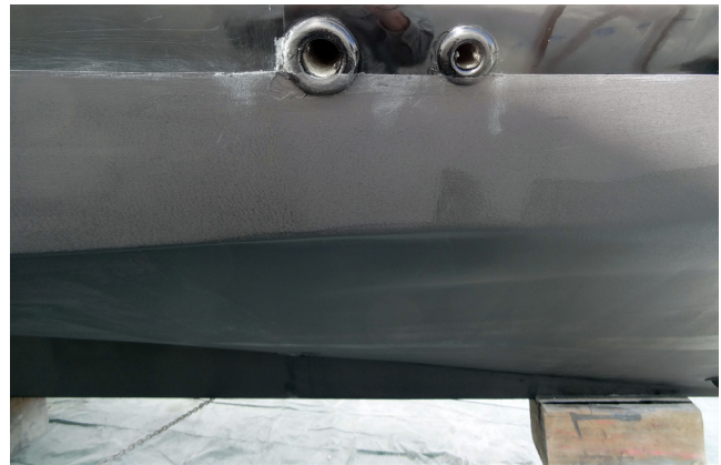
Finished chine transition from hard to rounded
