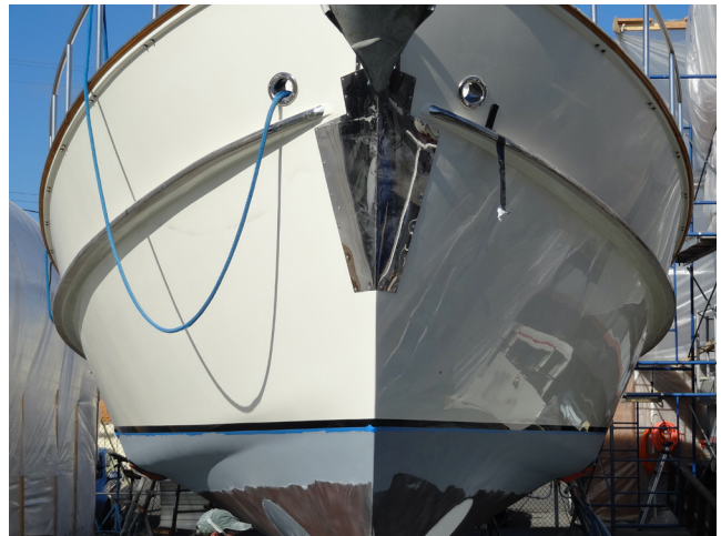
Rounded chine with epoxy barrier coat
